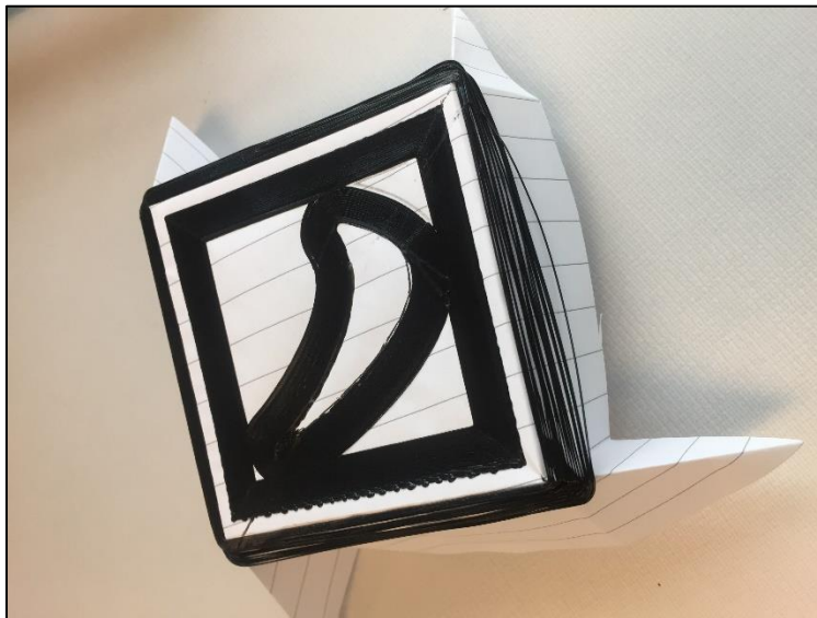
Fig 4-14: Sheet of paper used for collecting support material for upper part print
