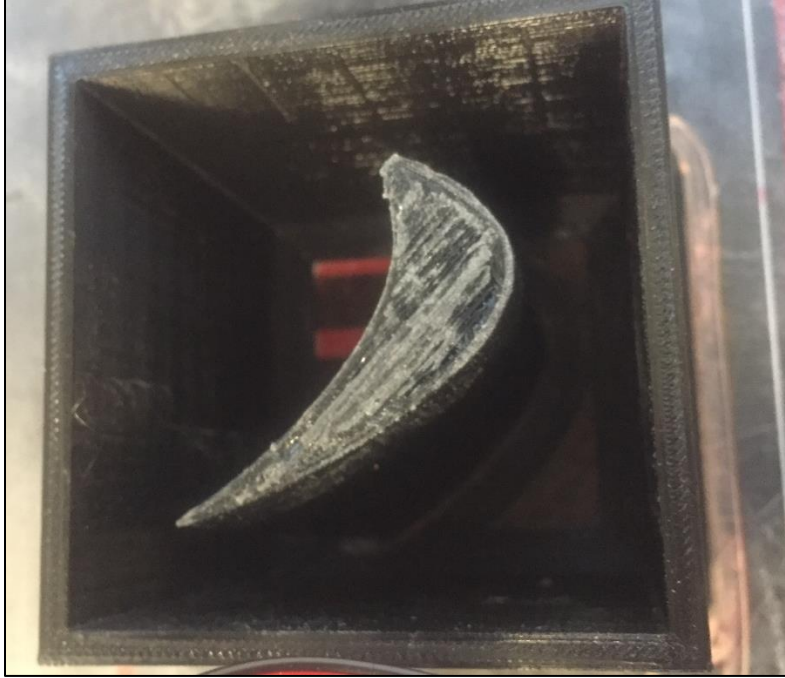
Fig 4-10: 3D printed lower part of turbine blade along with reference frame
