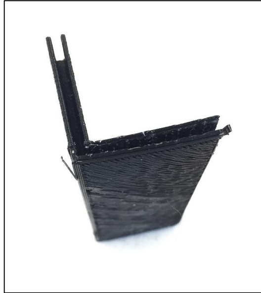
Fig 4-12: 3D printed V-block to offset the Z-axis
